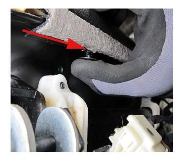
19. Insert two (5/16" stem diameter; 5/8" stem length) push pin retainers, GM P/N 00332364 or the equivalent, into the drilled holes from the underside as shown.
