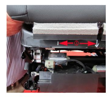
11. Measure 100 mm (4.0 in) on both sides of the center mark and mark the two locations with a paint pen (1).
