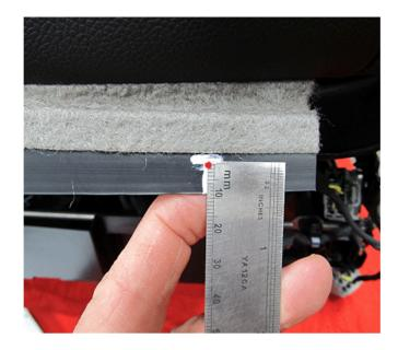
14. On the two seat cover mounting "J" channels, measure up 10 mm (0.25 in) from the lower edge and mark the location.
