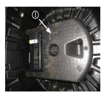
The tool (1) is stored in the foam container in the trunk, under the floor carpet.
