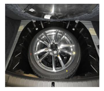
Open the spare tire lid and remove the spare tire.
