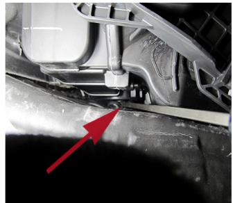
3. Reposition the seal using a flat-bladed tool as necessary. Inspect the drain assembly for the presence of a white or light blue plastic drain tube.
