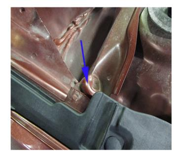
**Note:** It may be necessary to trim the excess body sealer in the plenum area to allow the seal to fit correctly.
