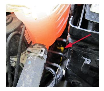
– Locate the first wire tie to the bracket directly below the coolant reservoir.
