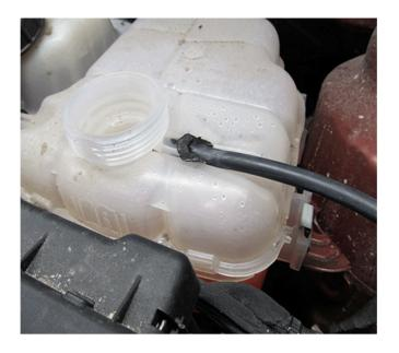
7.7. Insert the hose into the reservoir cavity as shown. Ensure the hose is fully inserted into the cavity and contacting the filler neck.
