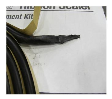
7.5. Stretch a small amount of butyl ribbon sealer, such as \*3M® Window Weld Ribbon Sealer, Part # 08612 or the equivalent, into a thin ribbon about 25 mm (1.0 in) in length as shown.
