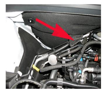
4. Inspect the plenum drain and ensure there is no foreign debris caught in the drain (leaves/twigs/pine tree needles) holding the cover open.
