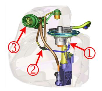
These connection are in the right side fuel tank Note the connections at the crossover pipe are not super easy to detect.
