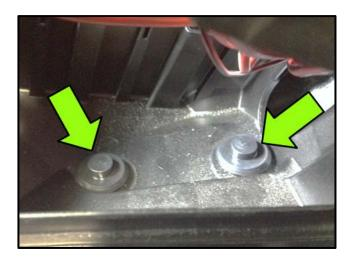
Install 1 plastic cap (N 910 706 01) onto each mounting nut <arrows>.
