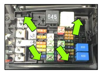
Reinstall the e-box into the housing and press firmly into position to make sure each tab <arrows> is seated fully into place.
