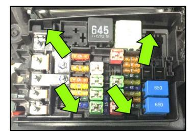
Release the tabs <arrows> while gently lifting the e-box upward out of the housing.
