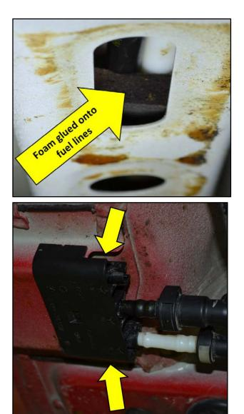
Adjust foam properly into Position 3 <as shown> and ensure the foam adheres to both fuel lines and fuel lines are not touching each other.
