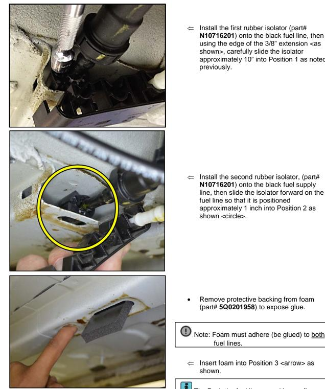
shown>, carefully slide the isolator approximately 10" into Position 1 as noted
