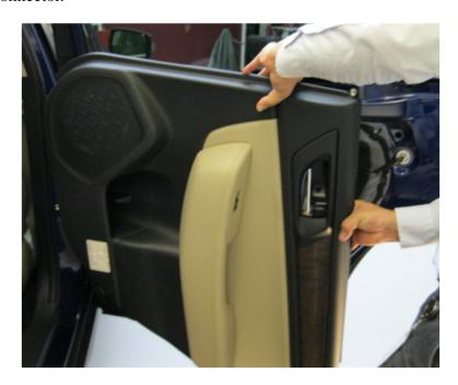
• After disconnecting the wiring harness connector for the power window and the speaker, put the trim panel in a safe place to protect it until needed.
