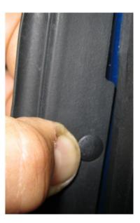
To complete this step, make sure the front of the weatherstrip is properly tucked in behind the chrome outer molding as shown below.
