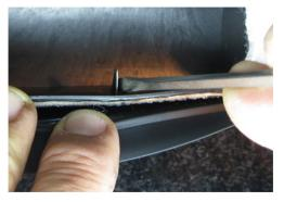
**CAUTION:** Wear Safety Glasses. Using an electric drill with a 5/32" drill bit turning at **LOW SPEED**, **CAREFULLY** drill out the two retaining rivets found between the "flaps" of the weatherstrip.
