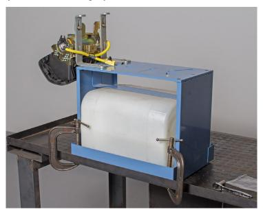
**STEP 2-** Remove the harness clip from the retainer bracket by rotating the harness / clip 90 degrees then releasing it from the bracket with needle-nose pliers.
