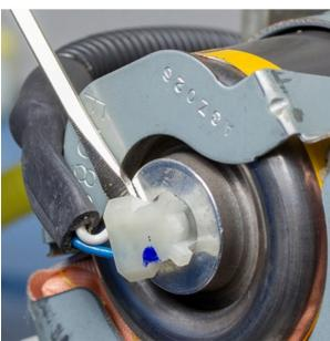
**STEP 12-** Refit the ends of the harness corrugated tubes to the retaining grooves of the mounting bracket as shown to complete the airbag module reassembly.
