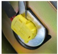
**STEP 12-** Reinstall the wiring harness retaining clip into its position on the mounting bracket.
