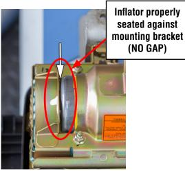
**STEP 10-** As shown below, install but do not fully tighten 2 of the NEW self-locking nuts while holding the stopper plate tight against the inflator. Remove the nuts still installed on the mounting bracket and replace them with 2 **NEW** self-locking nuts. Once all 4 **NEW** nuts are in place, torque to 31 - 38 inch pounds in the sequence shown below. Use a marker to mark the nuts after torquing indicating they have been fully tightened.
