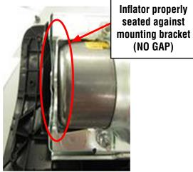
**STEP 10-** As shown below, install but **do not fully tighten** 2 of the NEW self-locking nuts while holding the stopper plate tight against the inflator. Remove the nuts still installed on the mounting bracket and replace them with 2 **NEW** self-locking nuts. Once all 4 **NEW** nuts are in place, **torque to 31 - 38 inch pounds in the sequence shown below**. Use a marker to mark the nuts after torquing to indicate they have been fully tightened.
