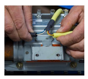
**STEP 3-** <u>CAREFULLY</u> cut the yellow harness cover (approximately 1 1/2 inches) enough to expose the 2 yellow and red wires inside and provide enough room to install the Electro-Tap (shorting) connector using a scissor or wire cutter (no knives or razors).
