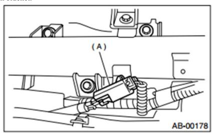
• Remove the 3 retaining bolts and **CAREFULLY** remove the airbag module from the vehicle and place it on a clean cloth to protect the dash trim outer surface portion from damage.
