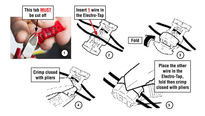
**STEP 5-** Once the Electro-Tap connector is fully crimped in place, cut the yellow and red wires on the **body harness connector side** of the Electro-Tap connector as shown below.
