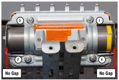
STEP 9- Once all 4 NEW nuts are in place, torque to 31 - 38 inch pounds in the sequence **shown above.** Use a marker to mark the nuts after torquing to indicate they have been fully tightened.
