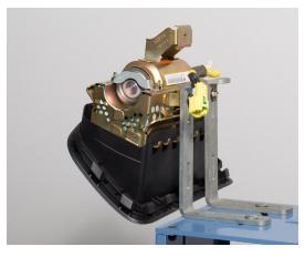
**STEP 2-** Peel the Sponge Tape and remove the harness clip from the retainer bracket by pushing the tangs inward with a flat-blade screwdriver as shown below. Always remove any Sponge Tape adhesive residue from the airbag mounting bracket using mild solvent on a clean shop cloth. **CAUTION:** Never use any silicone-based products for this purpose.
