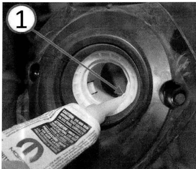
Fig. 7 Apply White Lithium To Outer Bearing Sleeve
