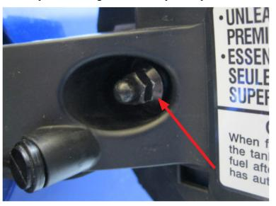
• Using a plastic trim tool, CAREFULLY work the trim tool in between the inner plastic filler door and the metal outer panel to release the 2 upper retaining clips. Once the upper 2 clips are released, the outer panel will be easy to remove from the door. A photo of the inner door with the outer panel removed showing the 4 clip locations is provided below to use as a reference.
