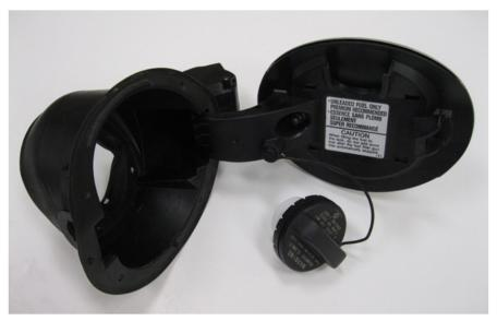
• Swap over the fuel cap / tether to the new saucer assembly. Release the tether retaining clip using a plastic trim tool as shown below.
