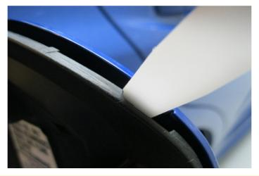
NOTE: Be careful not to drop or damage the outer panel while releasing the retaining clips.
