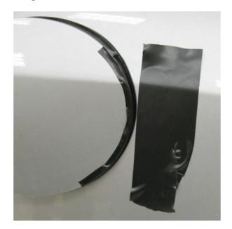
• Remove the fuel filler pipe protector (lock ring) by turning it CLOCKWISE.
