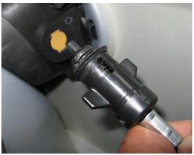
• Using a trim clip removal tool (or equivalent), pry up and remove the ring clip surrounding the fuel filler neck. There are 4 clips securing the ring clip. This part is a one-time use item as it will be broken during removal as shown in the photo below. **REMINDER:** Always take proper precautions to protect the vehicle's finish.
