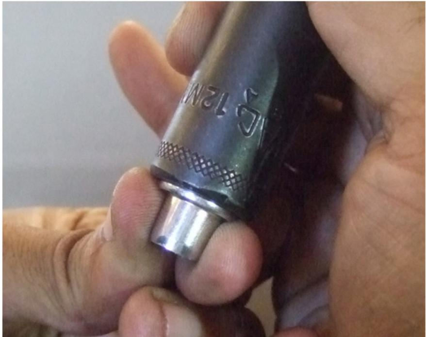
**NOTE:** The new breather vent assembly is also installed “dry” with **NO SEALER**. **CAREFULLY** tap the new breather vent into the cover while keeping the **impact** socket (installation tool) square and perpendicular as shown in the photos below. The tapping sound will change when the flange portion of the breather vent bottoms out and is fully seated (no gap) against the rear cover.
