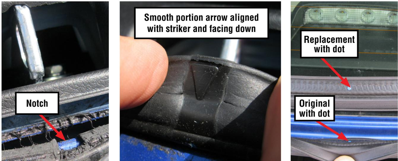
**STEP 3:** After the trunk stoppers (and weatherstrip on STI models ONLY) have been installed, close the trunk lid while paying close attention to the points listed below.
