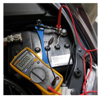
On vehicles with a battery sensor on the negative battery terminal, leave the terminal connected and connect a jumper lead to the bus bar area between the terminal end and the 12mm nut as shown below for the feed to the DVOM. Once the DVOM is connected, remove the 12mm nut, the battery cable from the stud then perform the test. After testing, re-torque the nut to 7.5 Nm (5.5 ft. lbs.).
