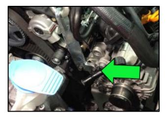
Install T10339 engine support bracket in place of the serpentine belt tensioner as shown <arrow>.
