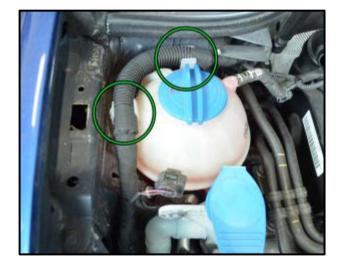
• Reinstall the turbo recirculation hose as onto the turbo inlet pipe as shown and reposition the retaining clamp <1>.
