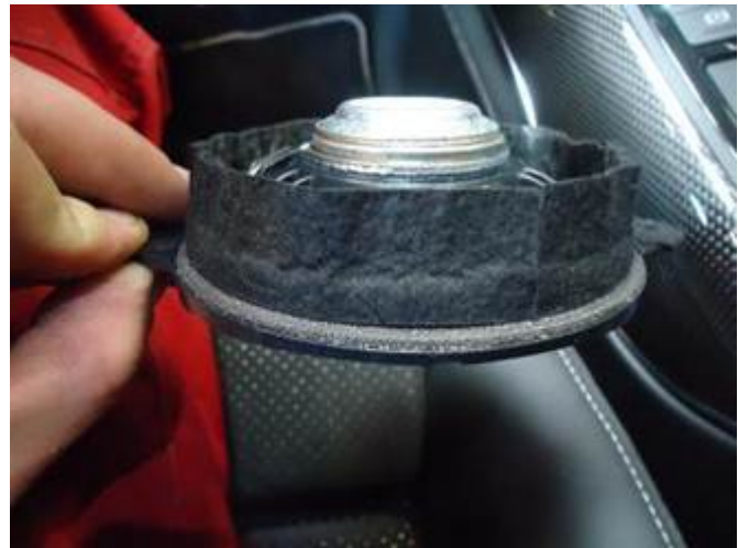
Figure 4. Center speaker with felt tape applied.
