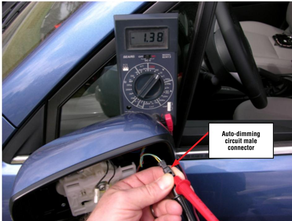
Once the Auto Dim circuit voltage is verified as acceptable, replace both exterior Auto Dim mirror glass assemblies following the procedure in the Accessory Installation Guide referenced above.
