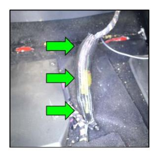
← Reinsert the airbag wiring circuit through the mesh wiring loom <arrows>.
