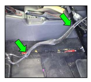
the mesh wiring loom <arrows>.
