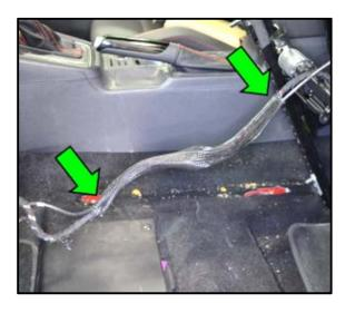
← If present, remove the tie wraps from each end of the mesh wiring loom <arrows>.
