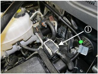
**Tip:** Shown in the graphic above, for easier access to the positive battery cable fastener at the junction box, disconnect the X121 connector (1).
