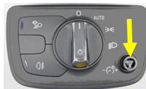
Figure 1. Control knob with missing cap
