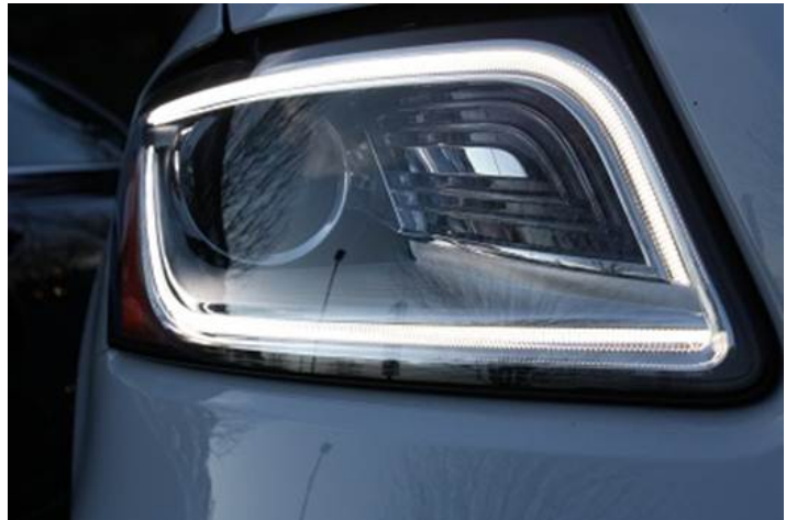
Figure 1. Upper and Lower light pipes illuminated.
