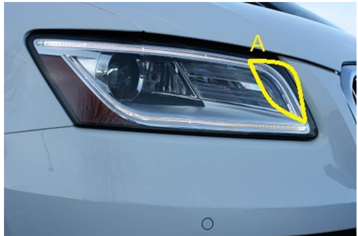
Figure 5. Upper light pipe perceived defect (A).
