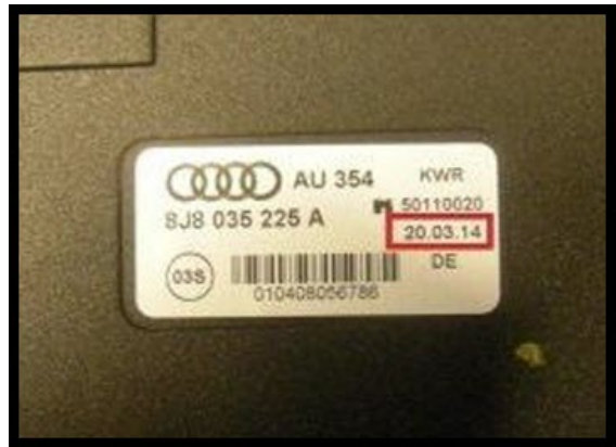
Figure 4: Manufacturing date on the aerial amplifier part label.
