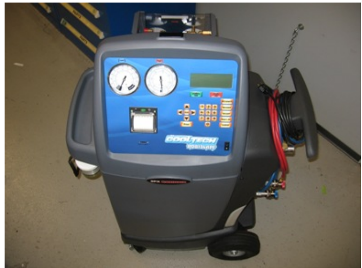
Figure 1. The ROB134APF Air Conditioning Service System with VAS 6337/1A Air Conditioning System Flushing Device.
