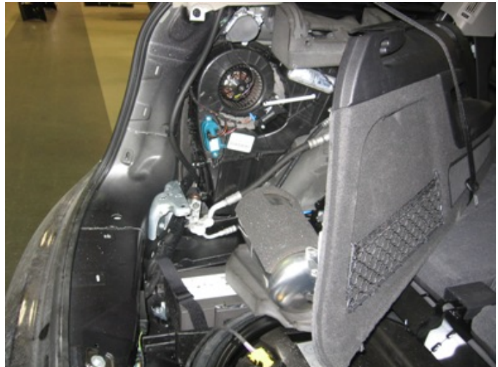
Figure 9. Location of rear air conditioning unit and expansion valve.
