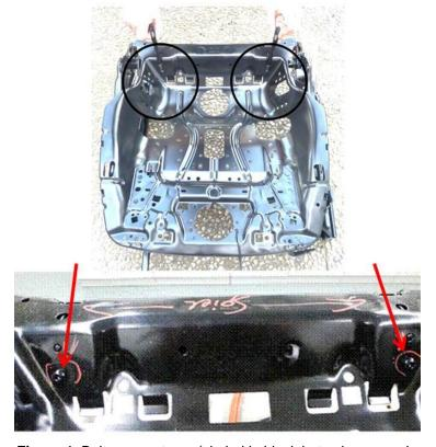
**Figure 1.** Bolts on seat pan (circled in black in top image and at red arrows in bottom image).
