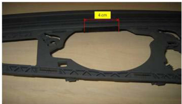
Figure 2. The felt tape should be applied to the area of the center defroster vent shown in red.
