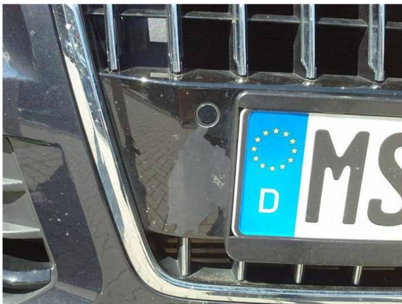
Figure 1. Example of flaked-off paint.
