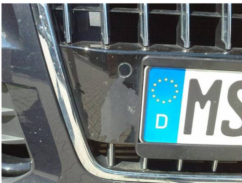
Figure 1. Example of flaked-off paint.
