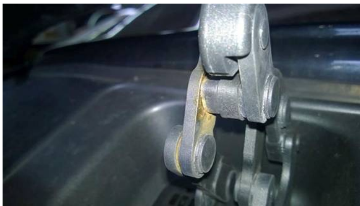
Figure 1. Corrosion on the spoiler drive unit hinge.
