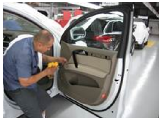
Figure 1. Removing the front door panel.
