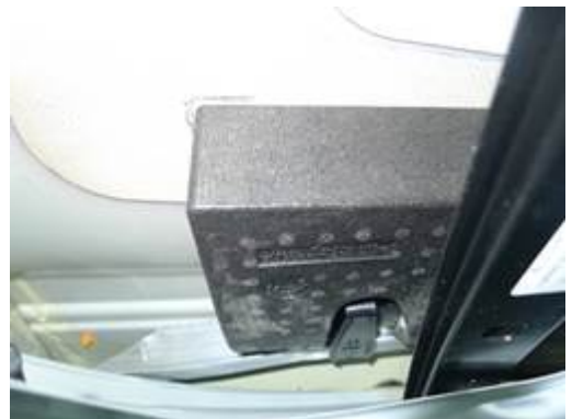
Figure 15. Lower pad installed to the correct position.
