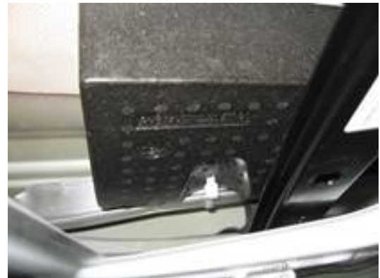
Figure 3. Lower pad secured to impact beam.
