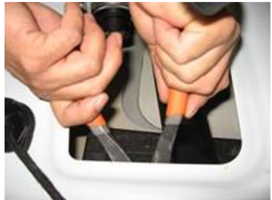
Figure 5. Cutting the retaining zip tie.
