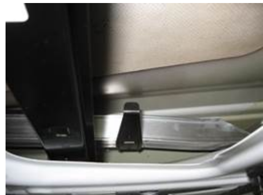
Figure 13. Retaining bracket installed on the impact beam.
