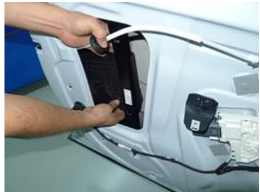
Figure 14. Reinstalling the lower pad.
