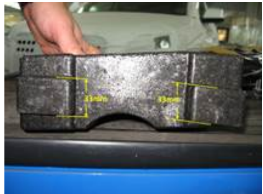
Figure 8. Pad legs with an original width of 33mm.
