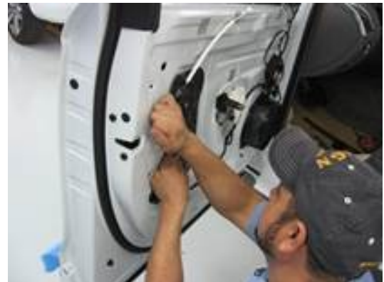
Figure 2. Removing the inner door panel cover.
