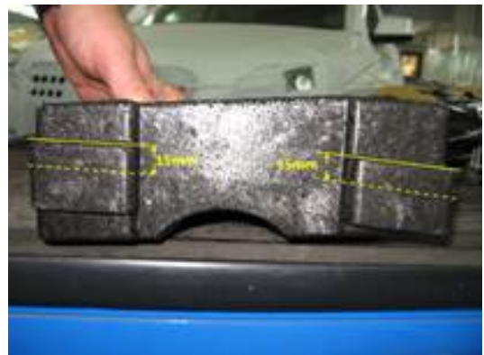
Figure 9. 15mm section of the pad legs to be removed.
