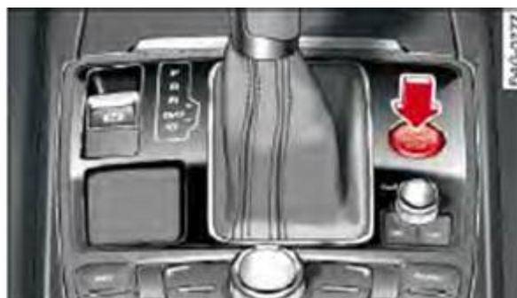
Figure 1. "START ENGINE STOP" button in center console.
