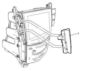
1. Remove the hazard warning switch. Refer to Hazard Warning Switch Replacement in SI.
