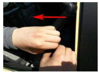
3. Pull the door weather strip to rework position.
