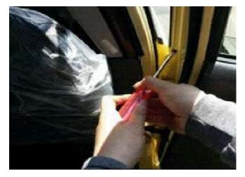
1.1. Lower the door glass window fully and remove the screw from door glass molding (located in interior door jamb) with screwdriver. (FRT LH/RH, RR LH/RH)
