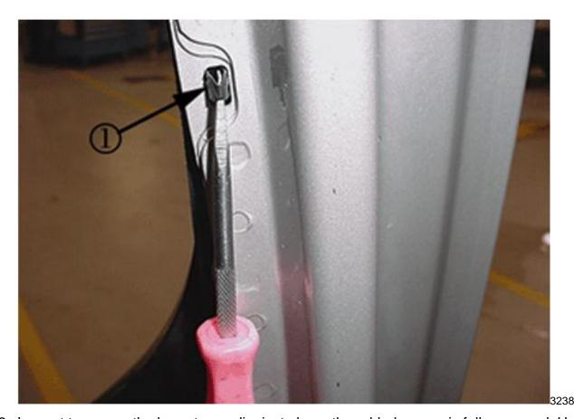
12. Inspect to ensure the lowest rear clip, just above the added spacer is fully engaged. Use a small screwdriver or hook if necessary (1).
