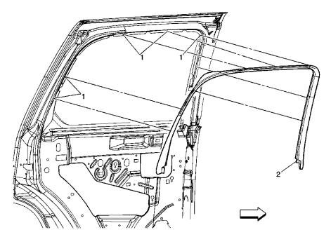
13. Carefully insert the lower ends of the rear door opening garnish molding behind the door trim panel. Line up the retaining points and carefully work the garnish molding into position and secure in place.
