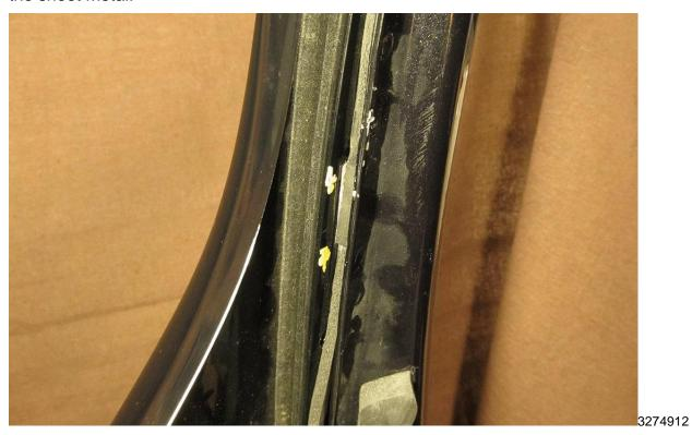
8. Remove the trim stick and apply pressure to the reveal molding adjacent to the spacer to ensure proper wet out.
