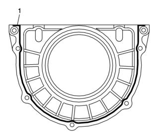
25. Apply a 3 mm (0.118 in) bead of RTV sealant (1) to the **NEW** crankshaft rear oil seal housing.
