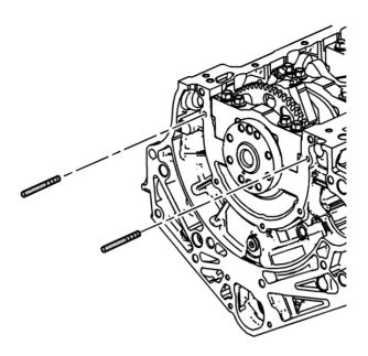
23. Install the 6 mm (0.236 in) guides from the *EN-46109 Guide Pin Set* into the 2 crankshaft rear oil seal housing corner bolt holes of the engine block.
