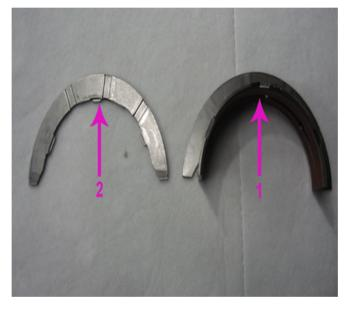
5. Typical view of a good crankshaft #3 thrust bearing with both thrust wings in place and a view of the crankshaft #3 thrust bearing (1) with one wing (2) broken off. The thrust bearing wing (2) is usually found in the engine oil pan, sometimes under the oil pan scraper. Ensure the failed thrust bearing wing is removed from the engine oil pan.
