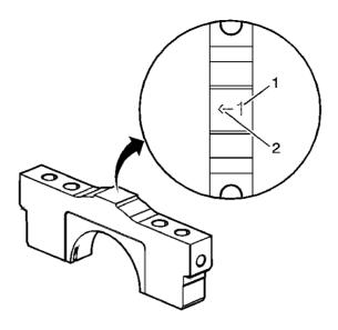
13. Install the main bearing cap with the arrow pointing towards the front of the engine.
