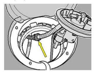
Figure 3. Fuel line connected to the locking flange.
