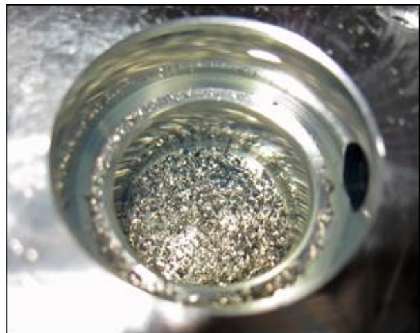
Figure 4. Example of a clear picture showing the metallic particles in the valve bore.
