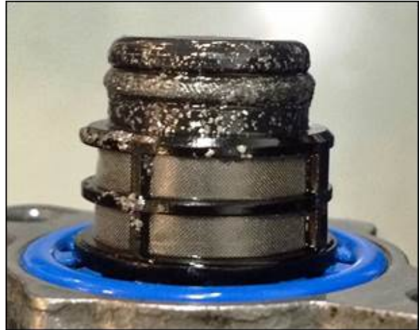
Figure 3. Example of a clear picture showing the metallic particles in the N290 fuel metering valve.
