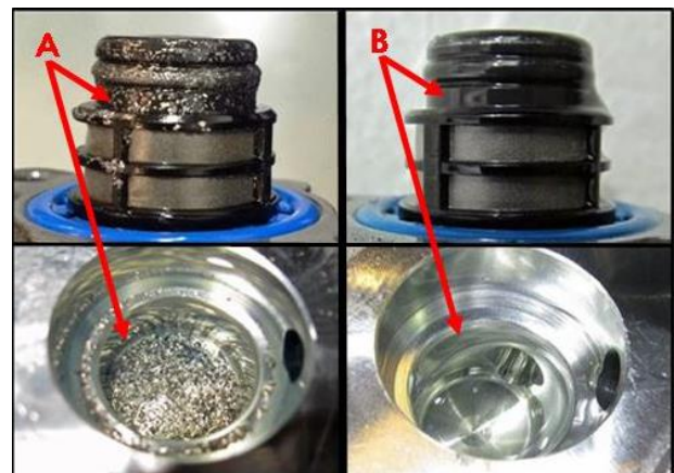
Figure 2. Fuel metering valve and valve bore with metallic particles (A), and without metallic particles (B).
