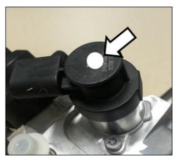
Figure 6. White dot on N290 fuel metering valve.
