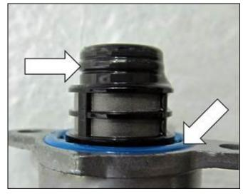
Figure 5. N290 fuel metering valve O-rings.
