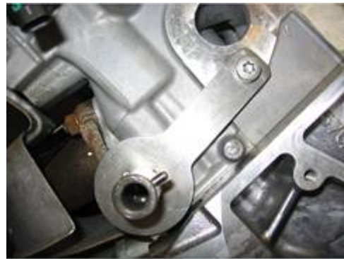
Figure 13. Engine adaptor on bank one.
