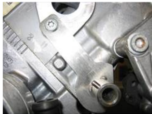
Figure 14. Engine adaptor on bank two.
