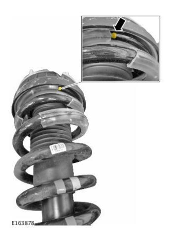
**3.** Using a suitable marker, make an alignment mark through the spring, packer and shock absorber.
