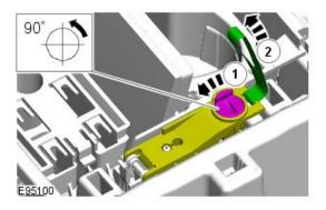
4. Disengage the parking brake.
