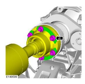
7. NOTE: Retain the locators for use with the new retaining bolts.
