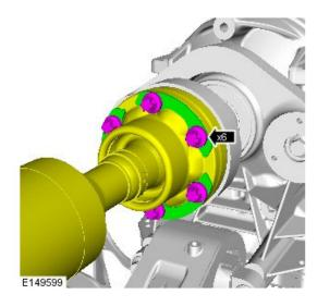
9. NOTE: Retain the locators for use with the new retaining bolts.
