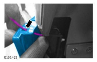
**13.** Locate the rocker panel moulding onto the location bracket and pull the cable tie tight.
