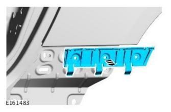
**6.** Using a suitable drill, drill out an 8mm hole in the rocker panel mounting bracket
