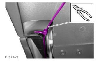
15. Visual inspection of the fitted cable tie
