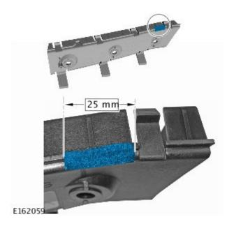
9. Install the rocker panel mounting bracket.
