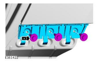
**5.** Remove the rocker panel moulding bracket.
