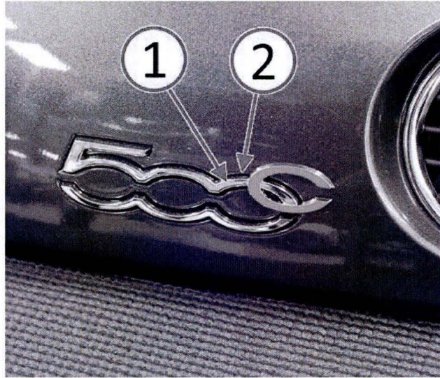
Fig. 7 Inspect Name Plate Alignment
