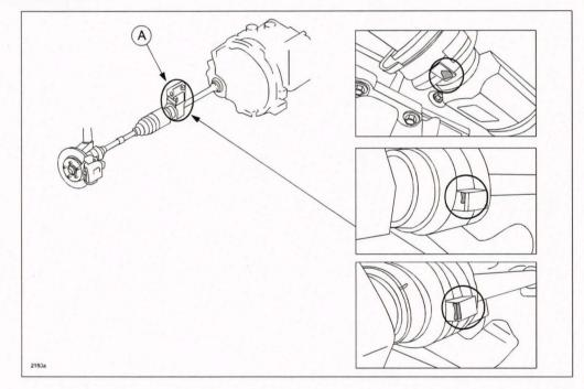
There is no functional problem with this issue since the amount of oil seepage is very small compared to the amount of grease. Note that the oil seepage will stop while the vehicle is in use.
