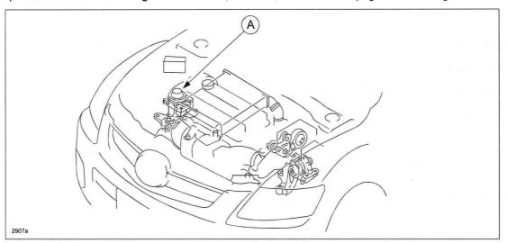
The engine mount rubber uses a new type of lubricant to eliminate this concern.
