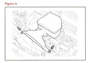
4. For PZEV vehicles: Remove the air cleaner cap sub-assembly.
