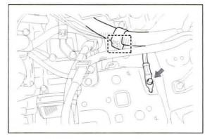
B. Remove the bolt and separate the ground cable.
