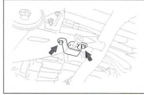
C. Remove the 2 nuts and bracket.
