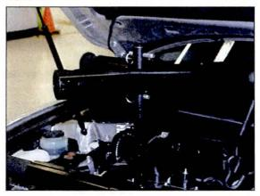
G. Adjust the height of the crossbar so it is level and insert the quick release pin through the nearest open slot in the straddle bar.
