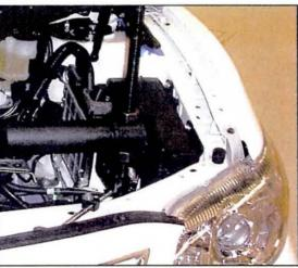
D. Place the front bar on the vehicle with the legs sitting firmly on the right and left frame rails near the radiator support, and secure the front bar arms to the radiator core support.
