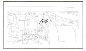
D. Loosen the hose clamp and disconnect the hose.
