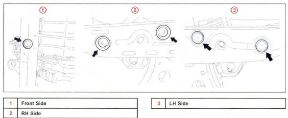
B. Remove the 9 nuts, and separate the front frame assembly.
