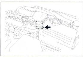
F. Remove the 2 bolts and the air cleaner cap sub-assembly.
