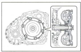
B. Engage the splines of the stator shaft and the stator while turning the torque converter clutch assembly.
