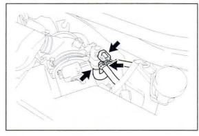
C. Separate the hose from the air cleaner cap sub-assembly.
