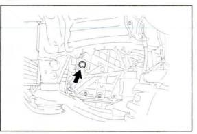
G. Install the refill plug. Torque: 49 N\*m (500 kgf\*cm, 36 ft\*lbf)
