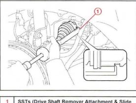
SSTs (Drive Shaft Remover Attachment & Slide Hammer [5 lb.])
