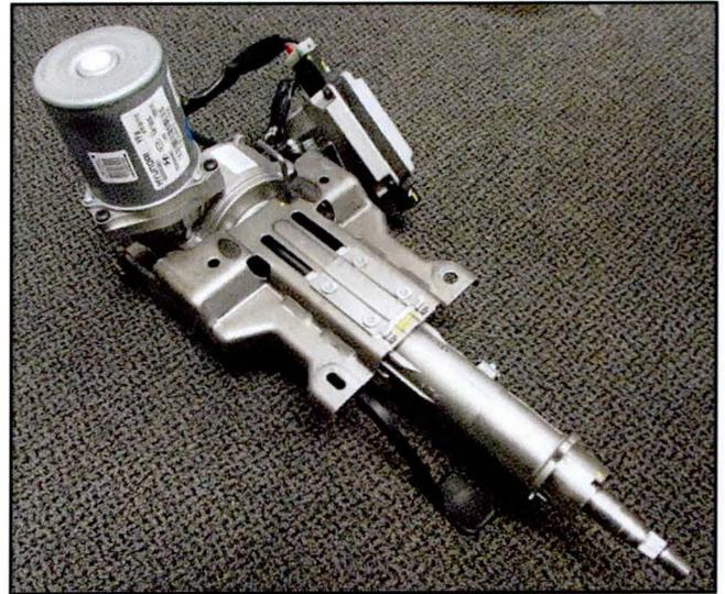
2. Loosen the 3 bolts (A) to remove the MDPS motor using a T25 socket, or similar tool.
