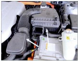
7. Disconnect the connector to the extension motor wire and temperature sensor.
