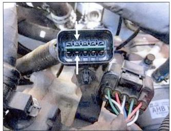
9. Disconnect the extension motor wire connector to the temperature sensor at the transaxle.
