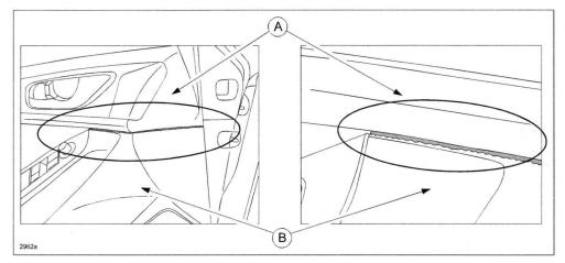
The cause of this is that the color of the felt and the glue is not appropriate and highly visible. To correct the problem, the color of the felt and the glue has been changed to one that resembles the door trim. The production control and the inspection have also been improved to eliminate the protruding felt.
