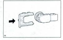
(a) Install the No. 2 ultrasonic sensor retainer as shown in the illustration.
