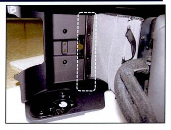
12. Remove the screws and then disconnect the connectors.
