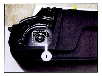
8. Remove the armrest frame (J) mounting bolts (white rectangle) and then remove the clips (white arrow)
